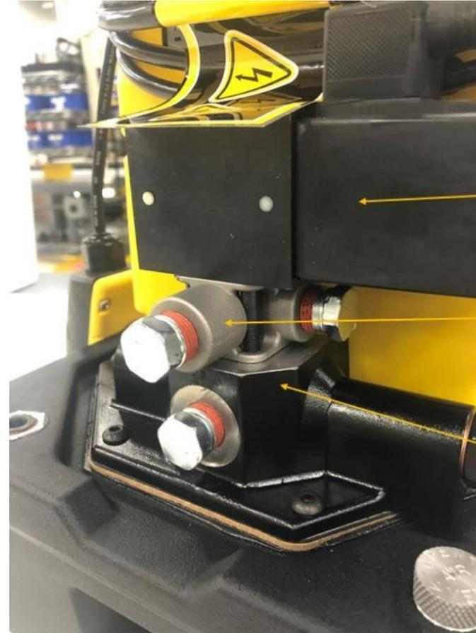
Steel Printed Manifold Installed on Enerpac Economy Pump – Close Up
